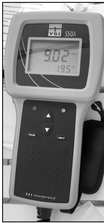
Left: This is the turbidity reader. We use it to test the turbidity level in the water. In the glass vile is an example of perfectly clean, non-turbid water. Center: This is the DO meter. We use it to measure the dissolved oxygen in the water. Right: This is the pH meter. We use it to measure whether the water is hard or soft
