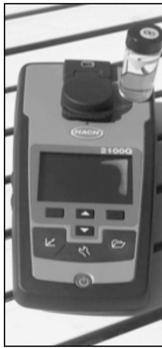
Left: This is the turbidity reader. We use it to test the turbidity level in the water. In the glass vile is an example of perfectly clean, non-turbid water. Center: This is the DO meter. We use it to measure the dissolved oxygen in the water. Right: This is the pH meter. We use it to measure whether the water is hard or soft
